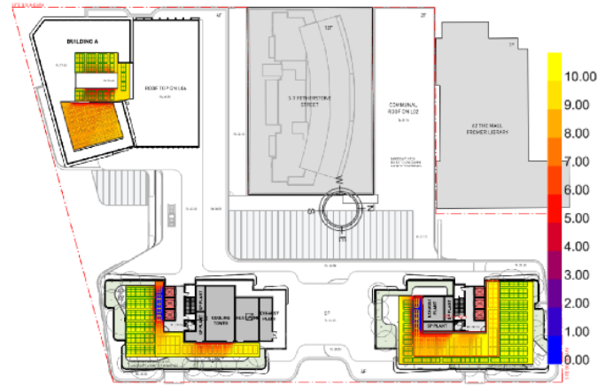
Figure 5.7 Roof solar exposure - winter
